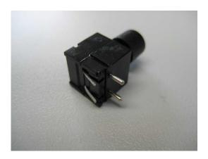
(6) With a small soldering iron it is possible to solder the two mounting bolts without extending the complete PCB from the chassis. Please take care to solder the two bolts quickly, because they are just press-fitted in the plastic body of the pushbutton. Connect the contacts on the rear side of the pushbutton also carefully with respect to the closed plastic housing.
